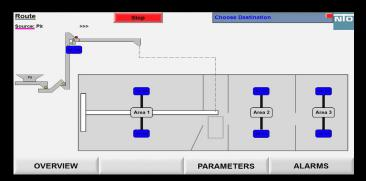
When the system is in manual mode, it is possible to start and stop motors and set their speed (if the motors are operated by frequency converters) manually. It is possible to view graphically on the screen which of the motors are running and which of them have stopped. For manual control of the cross conveyor, we recommend the option with an 8-function remote control.
